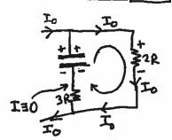
@ loop rule around RH loop (+Vco) + (-Io2R) + AV3R = 0
