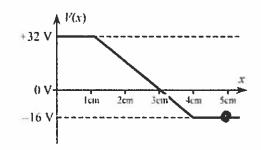
$$\overline{E}_{x} = -\frac{dV}{dx} = -\left(\text{slope of V-vs-x graph}\right)$$
