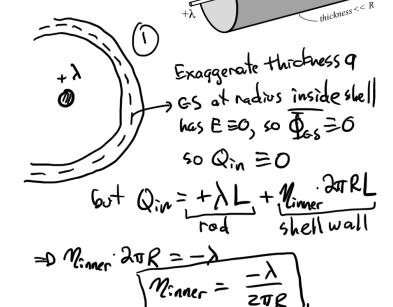
(2) Shell has charge/length+ $\lambda$ -> a length L has total charge Quel = + > L, split between inner and outer valls
