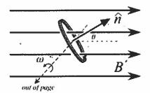
When loop is ariented with normal n making angle 0 with B-freld, flux is  $\Phi = \int \vec{B} \cdot d\vec{A} - \vec{B} \cdot \vec{A} = B \pi R^2 \cos\theta$
