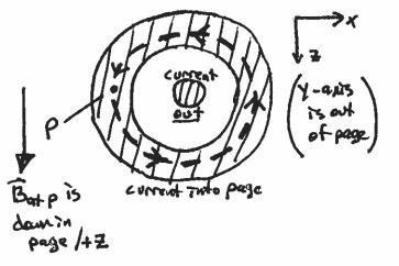
Apply Amperes Law: & B. ds = Mo I through Choose Amperian loop of radius 4R, passing through point P (dashed curve at left)
