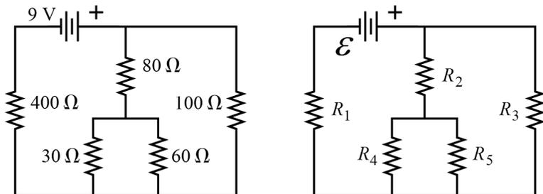
Find the equivalent resistance of the circuit. Resistors  $R_4$  and  $R_5$  are in parallel.
