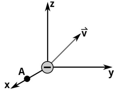
With  $\hat{r}$  in the  $+x$  direction, the Right-Hand-Rule shows us that  $\vec{v} \times \hat{r}$  is down and to the right on the page (positive  $y$  and negative  $z$ ). Since the particle is negative,  $q\vec{v} \times \hat{r}$  must be in the opposite direction, up and to the left on the page (negative  $y$  and positive  $z$ ). That direction is expressed by
