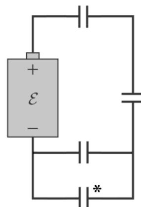
The top and right-most capacitors are in series (same charge). Their equivalent capacitance can be found.
