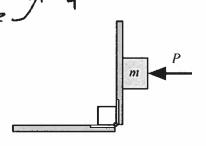
(i) Note block is about to slip, so we know that static friction -> max value
