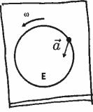
1 Moving ccw and slowing down —D tangential accel is opposite to motion
