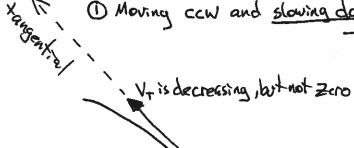
1 Non-zero tangential velocity requires radially inward acceleration component
