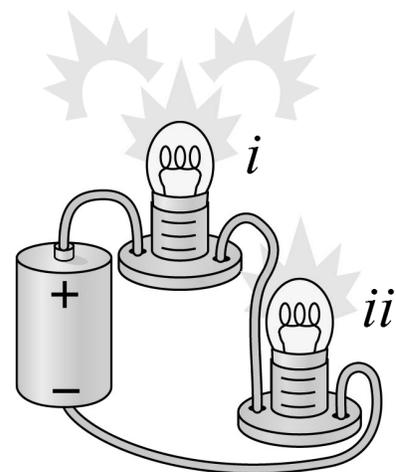
Reversing the polarity of the battery will change the direction current flows through the circuit, but does not affect the equivalent resistance of the circuit, so the current supplied by the battery does not change. The bulbs are in series, so that unchanged current passes through each bulb. With the same current flowing through the same bulbs, the brightnesses will be unchanged.
