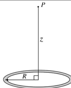
From symmetry considerations, the electric field must be directed along the  $z$  axis, so  $E = E_z$ . Using the relationship between field and potential,
