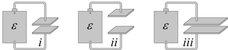
As the capacitors remain connected to their batteries, the potential across each capacitor remains constant, making  $U = \frac{1}{2} C (\Delta V)^2$  more useful.
