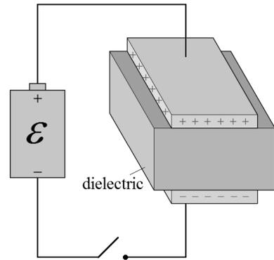
As the capacitor is disconnected from the battery when the external agent is removing the dielectric, the charge on the plates can't change. That charge is
