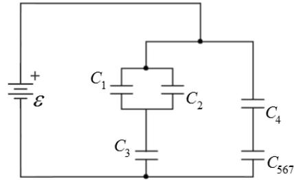
$$\begin{aligned} C_{4567} &= \left( \frac{1}{C_4} + \frac{1}{C_{567}} \right)^{-1} = \left( \frac{1}{C} + \frac{1}{3C} \right)^{-1} \\ &= \left( \frac{3}{3C} + \frac{1}{3C} \right)^{-1} = \left( \frac{4}{3C} \right)^{-1} = \frac{3C}{4} \end{aligned}$$
