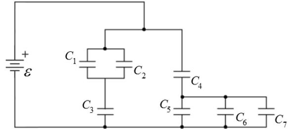
Combine capacitors in series or parallel until a charge on and potential across an equivalent capacitance can be determined. Then work back, finding charges and potentials on individual capacitors.
