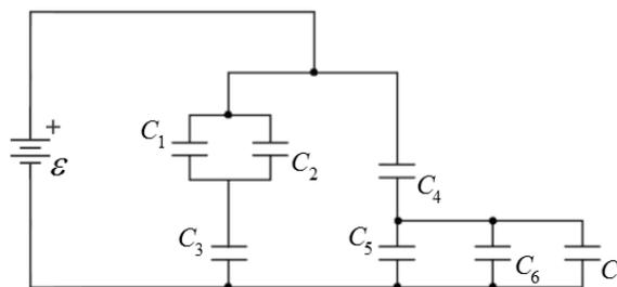
1. (6 points) Let your answer to the problem above be  $Q_7$ . If the emf of the battery were doubled, and the capacitance of all the capacitors was halved, what charge  $Q'_7$  would be on capacitor  $C_7$ ?
