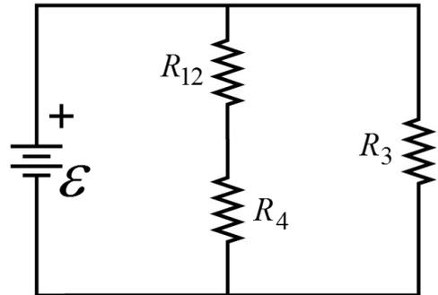
The potential across  $R_{12}$  can be determined from the definition of resistance,
