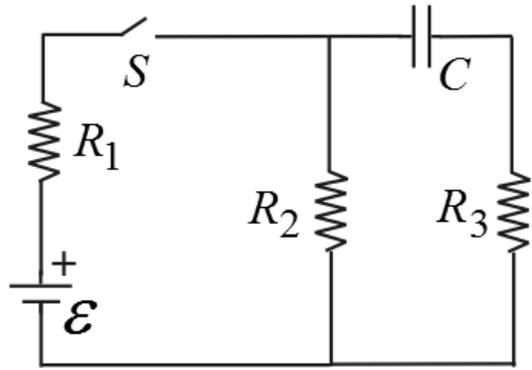
After the switch has been closed for a “very long” time, the capacitor will be fully charged. Therefore, there can be no current flowing in the branch with the capacitor (or else charge would be delivered to it, and it wouldn’t be fully charged). With no current flowing in the branch with the capacitor, there is no current flowing through resistor  $R_3$ , so the potential across  $R_3$  is zero, and the potential across the capacitor must be the same as that across resistor  $R_2$ .
