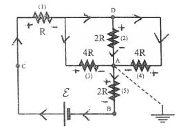
@ Nother that 1, (234), and 5 are in series Rier = R+R+2R = 4R = D Total current twough emf is found from simple loop + E-Inor Reg =0 | Inor = E |
