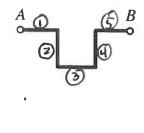
For all five segments, total length is Lin = 5L have, total resistance can be found by neglecting the 90° bends  $R_{TOT} = \frac{DL_{TOT}}{A} = \frac{DL}{A} = \frac{200L}{TLd^2}$
