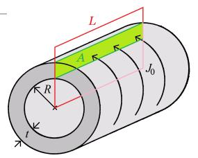
Use Ampere's Law. Choose a rectangular Amperian Loop of length L, with one side along the field line in the center of the cylinder, and the opposite side outside the cylinder (shown in red and pink).
