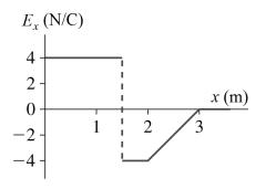
That is, the change in potential is the opposite of the area under the graph of field as a function of position.
