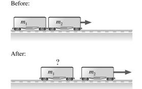
A system consisting of the railcars had no net external force on it. Momentum is conserved in that system.
