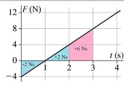
The area under this force-time curve from zero to t = 3.0 s is +6 N·s. Letting signs indicate directions in one dimension, .....
