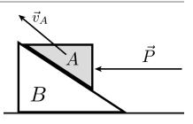
The normal force of A on B must be perpendicular to the surface between them. The friction force of A on B must be parallel to the surface between them.
