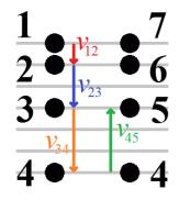
The average acceleration at time 4 is proportional to the velocity change  $\vec{v}_{45} + (-\vec{v}_{34})$ . In terms of the horizontal bar spacing,  $\vec{v}_{45}$  is three spaces up, and  $\vec{v}_{34}$  is three spaces down. The difference, six space up, is proportional to the average acceleration at time 4, and is of much greater magnitude than the acceleration while the ball is in free fall. The greatest acceleration magnitude occurs
