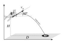
Determine the elapsed time that the bomb will be in flight before it hits the ground. What horizontal distance D should Buzz be in front of the "G" at the moment he releases the bomb? (Use  $g = 9.80 \text{ m/s}^2$ ).
