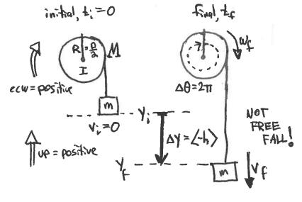
Assumptions - drag can be neglected, Friction too -cord is massless and unstretchable -cord unwinds from wheel without slipping & |DYwag = DSrord = RADwheel Vog = Voord = R Wuheel - acceleration is constant while unwinding
